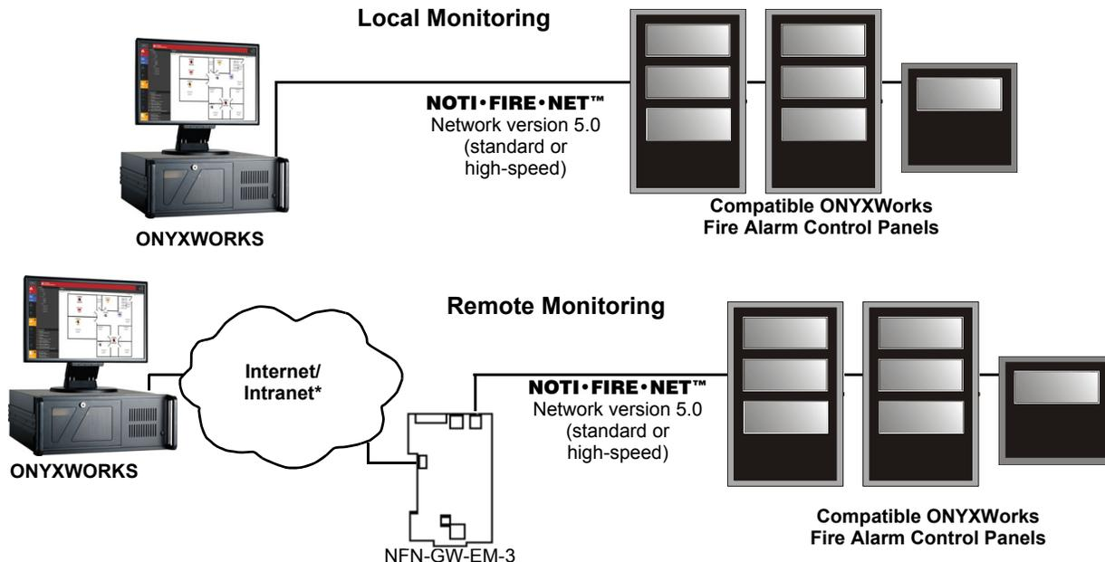
\* A UL Listed ethernet (TCP/IP) switch is required between a shared-IP network and the ONYXWorks equipment. Contemporary Control Systems, Inc. ([www.ctrlink.com](http://www.ctrlink.com)) has several UL864 recognized switching hubs.
